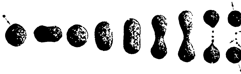
Fig. 24.3 Schematic representation of steps leading to the fission of a compound nucleus, according to the liquid drop model.
